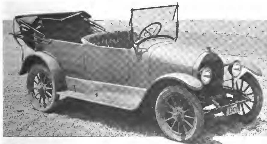
Left—Jeffery 1915 Chesterfield six with touring body. Note streamline design, flush doors and clean running board. Right—Rear view of the same car showing the accessible gasoline tank fillers and spare tire carrier hung directly on the rear of the frame members
